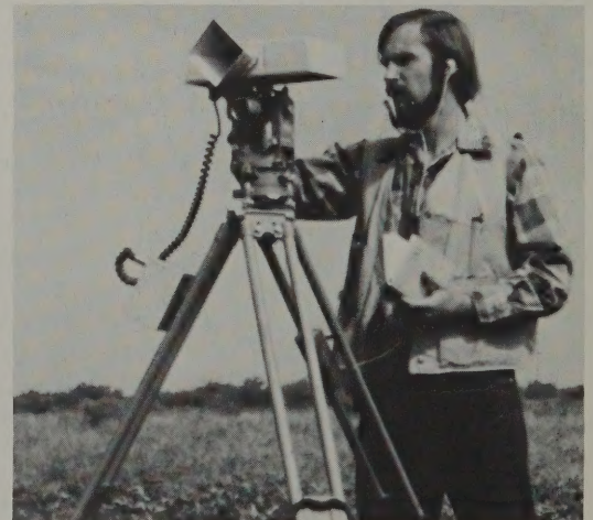
Electronic distance measuring equipment replaces link chains and steel tapes.
